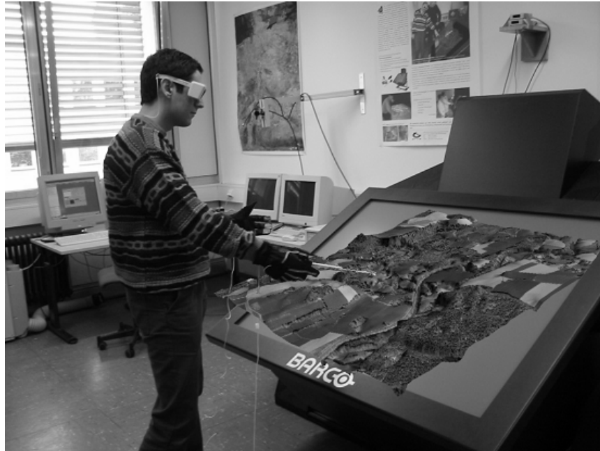
Figure 2: Semi-immersive Workbench that enable interaction within the virtual environment in order to 'plan' measures and investigate their impacts
